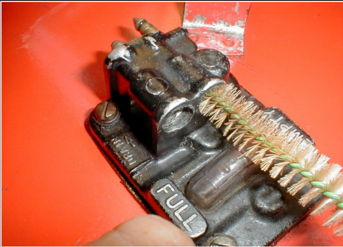
Illus #9 . Extract the core plug, pin and old o-ring from the air vent side. Clean both orifices well.
