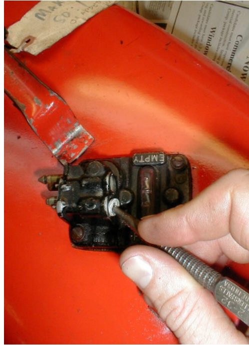
Illus #4. Use the punch to pop out the old core plug
