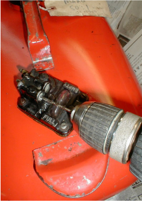
Illus #3. Dimple the core plug with a punch then use a 1/8" drill to make a hole. You only need to go through the core plug, don't go too deep!
