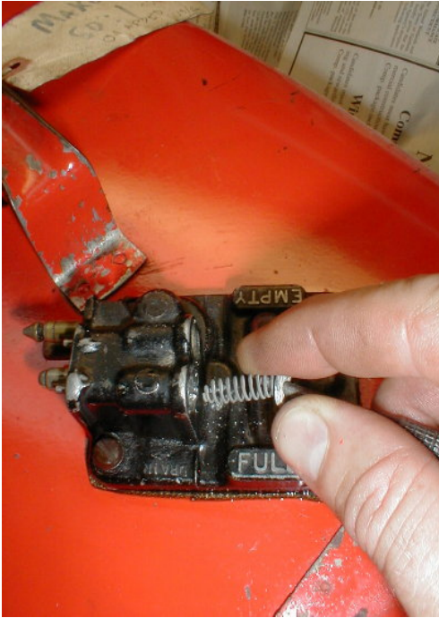
Illus #5. Remove the spring - note tapered end of spring goes in on reassembly
